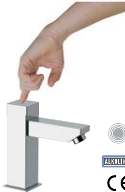
TTE 19 CR € 408,60 Electronic timing pillar tap with piezoelectric activation button, batteries powered, minimal squared shape, all in c.p. brass, opening time about 10 seconds, angle valve with filter included.
