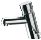
TE 18 M Temporized (timer) mixer pillar tap with hot/cold water selection handle, serie minimal. 1/2", in c.p. brass, opening time 6-8 seconds.
