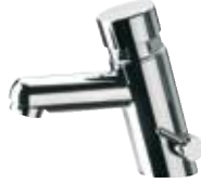
TE 19 M Temporized (timer) mixer with water mixing through headvalve, pillar tap with hot/cold water selection handle, serie minimal. 1/2", in c.p. brass, opening time 6-8 seconds.
