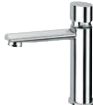
TE 22 Temporized tap 1/2", oval line all in Cp brass opening time 6-8 seconds.
