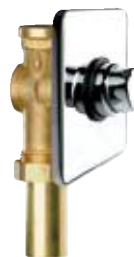
TE 171Q Temporized (timer) built-in squared tap for wc, 3/4, 1", opening time 6-8 seconds.
