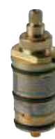
E 50 Thermostatic cartridge with 330° angular handle rotation, 38° safety lock, working field from 5°C to 80°C, pressure field from 1 to 10 bar, stainless steel filter and safety system with the outlet lock in case there is one water lock.
